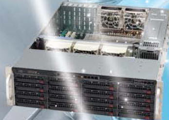
SC836/A/E1/E2/E16/E26 and SC836-JBOD 16 Hot-Swap HDDs in 3U
