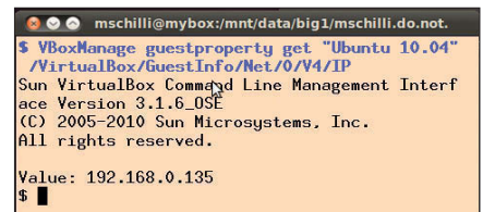
Figure 9: The guestproperty command shows you which IP address the specific virtual machine has picked up from the DHCP server.
