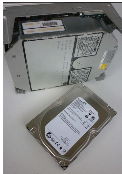
Figure 1: Old and new side by side: a physically large hard disk, with just 85MB capacity (background), and a state-of-the-art 3TB SATA hard disk by Seagate (foreground).
