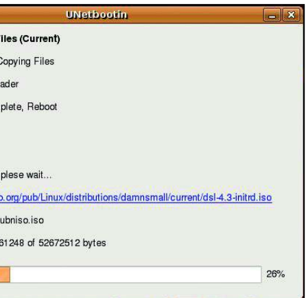
Figure 2: If you select a distribution the software supports, Unetbootin will retrieve it from an FTP server and install the distribution on your memory stick.
