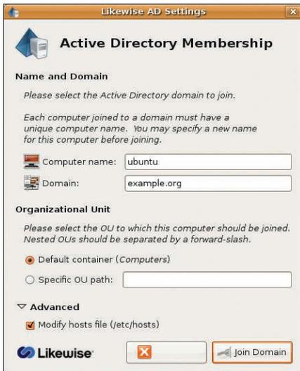
**Figure 3: The Likewise Open GUI expects the DNS name of the domain and the hostnames.**
