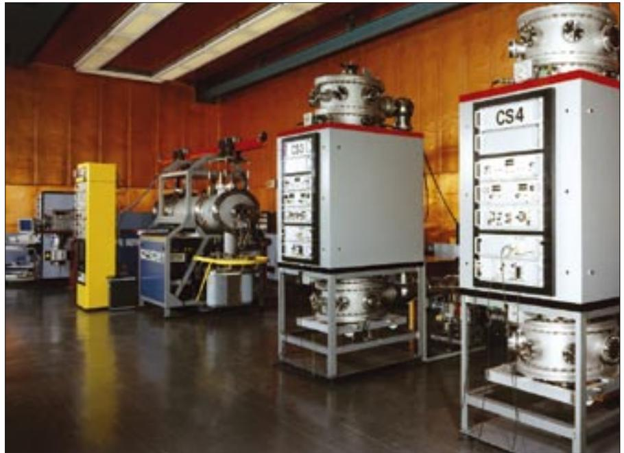
**Figure 1: The Physikalisch-Technische Bundesanstalt in Brunswick, Germany, has a number of atomic clocks. The clocks are accurate to about one to three billionths of a second per day, that is, about one millionth of a second per year. Computers on the Internet can use these clocks as time sources.**
