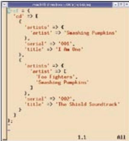
Figure 2: This is the data structure that XML::Simple uses to store the sample data.
