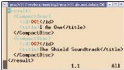
Figure 4: twigfilter outputting the modified XML.
