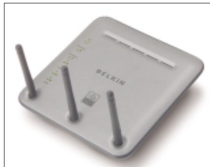
Figure 3: Some manufacturers have already started to offer "Pre-N" systems based on the MIMO principle. The Belkin router shown here achieves transfer rates of over 300 Mbps in the 2.4 GHz band.
