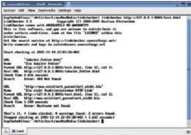
Figure 2: Finding faults: Linkchecker finds the errors in “test.html” with some help from the web server. The tool checks four links and reports that two are bad.
