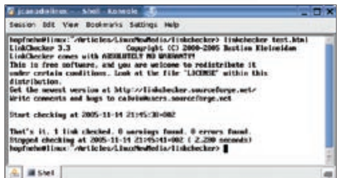
Figure 1: Linkchecker has problems with the filesystem. It ignores two errors and just tests one link.
