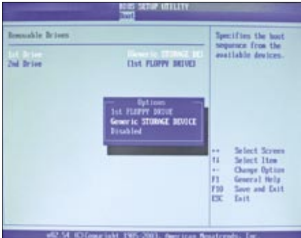
Figure 1: Booting from a USB stick - every BIOS does its own thing. Our sample BIOS refers to removable drives and a generic storage device.
