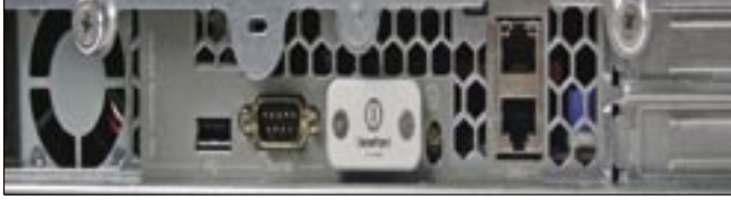
Figure 5: Ironport fits a cap to the VGA port; attaching a display is not an option.
