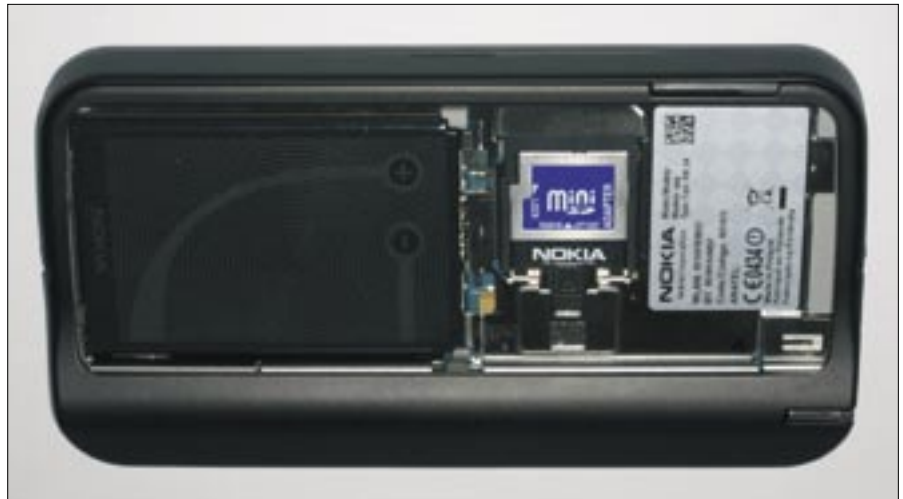
Figure 2: The Nokia N800 comes with a 128MB Micro SD card. A matching SD adapter integrates the card with the device.
