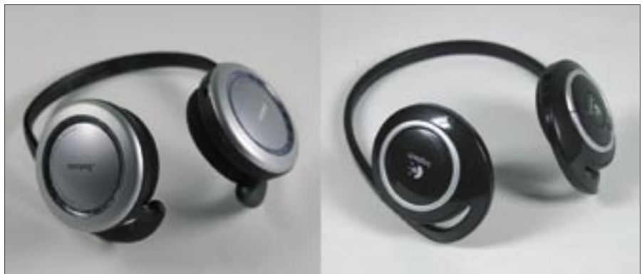
Figure 1: The Bluetooth headsets by Jabra (left) and Logitech (right) both support stereo sound. The Jabra headset also supports the mono SCO profile.
