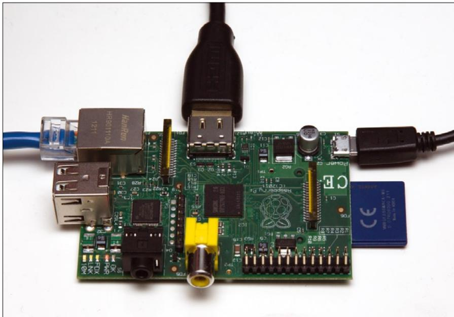
**Figure 1:** Raspberry Pi model B with two USB ports; one 10/100 Ethernet port; sound, HDMI, and composite ports; a number of freely programmable I/O hardware ports; and an SDHC memory card.
