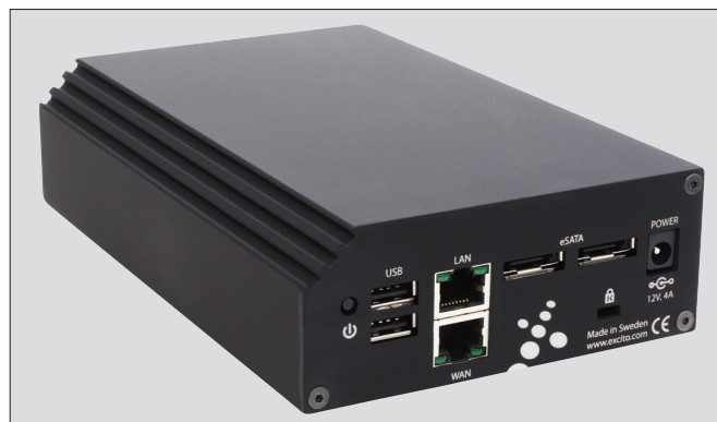
Figure 1: Bubba Two sports eSATA and USB ports as well as two Gigabit Ethernet jacks.
