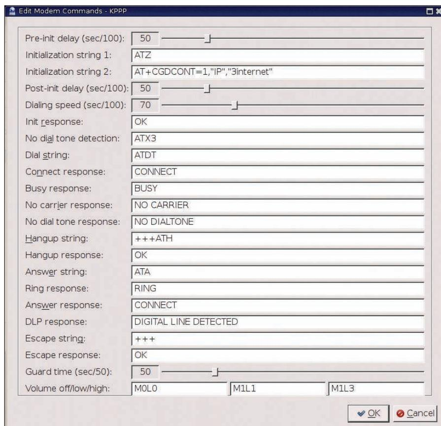
Figure 1: Configuring modem settings with *kppp*.
