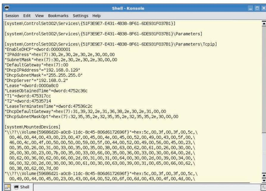
Figure 4: Dumphive converts the Windows Registry to cleartext. Search tools such as *grep* can then help you reconstruct critical settings, for example, the password hash or IP data.
