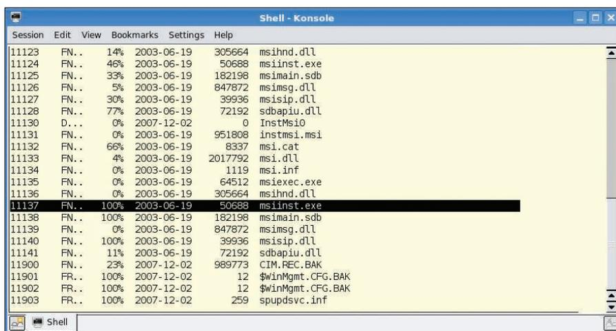
Figure 3: Ntfsundelete shows deleted files that can be undeleted. The first column contains the inode number required to restore the file on the filesystem in the image file.
