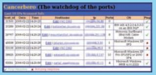
Figure 1: Cancerbero's detail view after completing a scan. The PHP front-end lists the open ports and the operating systems of the servers.
