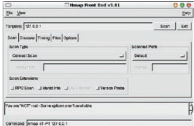
Figure 3: Without root privileges, Nmap is restricted to a small selection of techniques for identifying open ports across a network.
