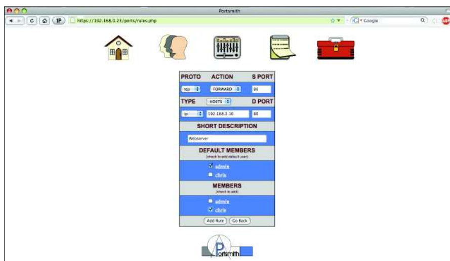
Figure 2: Modifying the ruleset: The example forwards port 80 on the firewall to an internal web server.
