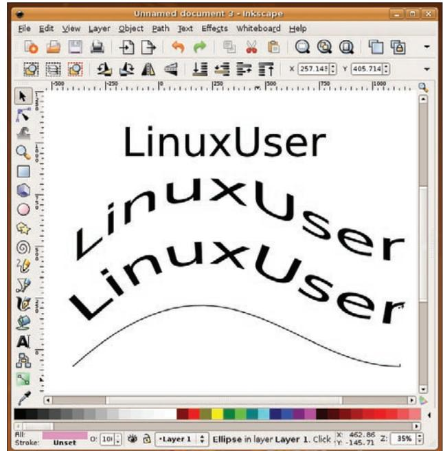
Figure 5: Amazing text effects with a minimum of effort: The original text is shown at the top; the path on which it was aligned is at the bottom. In between lie the text that was modified with the Ribbon option (above) and the text modified by the Snake option (below), both aligned along the path.
