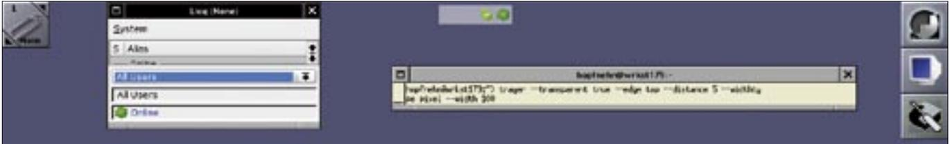
Figure 2: Command line options help users specify the screen position and transparency mode for Trayer.
