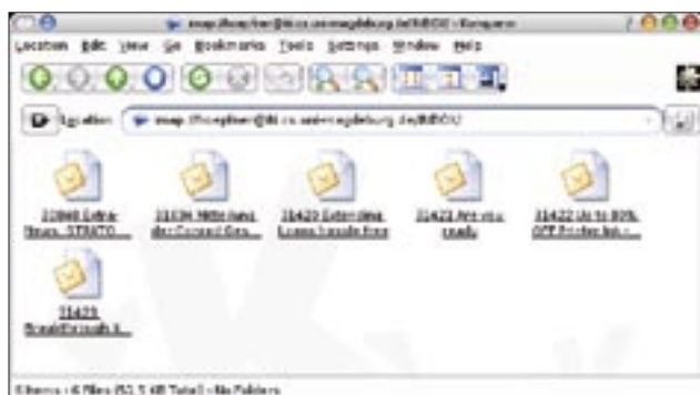
Figure 5: The imap kioslave lets you remove a mailbox as you would a local directory.
