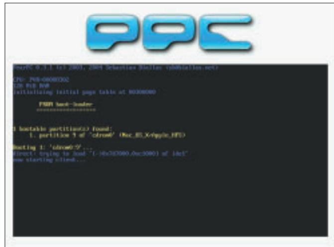
Figure 3: The PearPC start screen allows you to select the boot partition.
