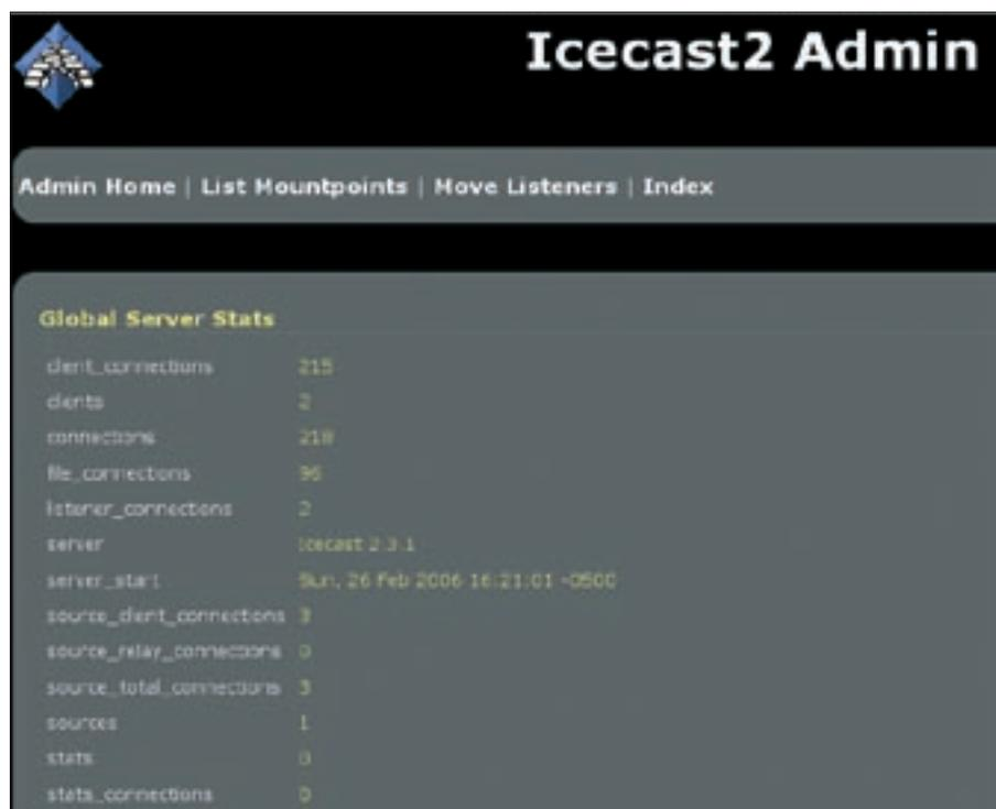
**Figure 4:** Administration is easy with the Icecast web interface. Use the Global Server Stats page to check the current status of the server.
