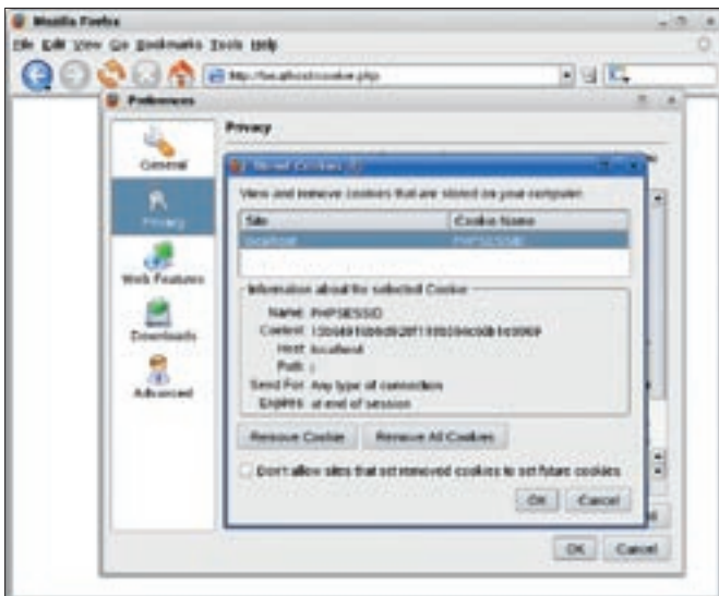
Figure 4: Web applications use cookies to identify users. If attackers can access these credentials via cross-site scripting, they can steal your identity.
