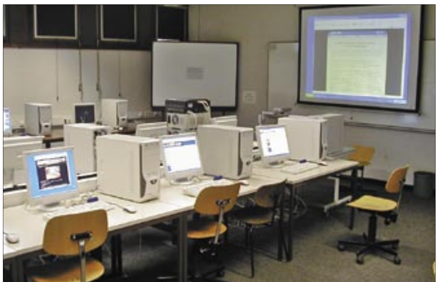
Figure 1: The machines in the CIP pool are set up as diskless clients. To avoid overloading the network at boot time, we dug deep into our box of tricks and replaced the network filesystem with remote block devices.
