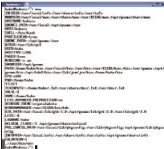
Figure 1: Everything is variable - "env" outputs a complete list of Bash environmental variables.
