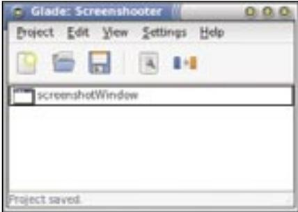
**Figure 1: The project window lists all of the top-level windows and dialogs included in the current Glade project.**
