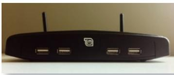
ment, “the hardware is unique, and the box and form-factor are amazing.” The unit features a die-cast solid-metal case, which acts as a passive heat sink. The device cools its components without needing fans, so it’s almost silent.
