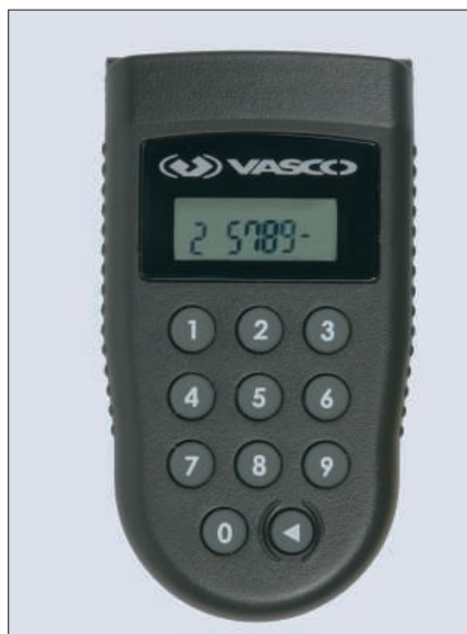
Figure 1: The Digipass Pro 300 by Vasco relies on the challenge-response approach. The user types the challenge via the keypad on the token and reads off the response from the display.
