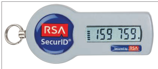
Figure 2: The Secur-ID-Token SID700 by RSA/EMC encodes the current time of day and the internal key. The display shows a different PIN every minute.
