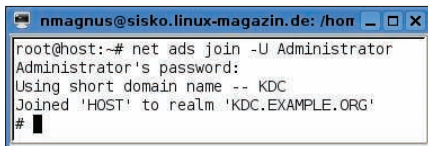
Figure 4: To add the local machine as a member of the standard domain, the user on the domain controller (DC) needs administrative privileges. After entering the password, the DC adds the new client to the domain.
