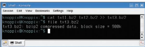
**Figure 1: Follow the standard procedure to concatenate compressed files with the cat command.**
