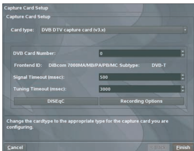
Figure 4: Immediately after we set the "Card types," the DVB-T USB stick plugged into the machine was detected. In this case, no other settings were needed.
