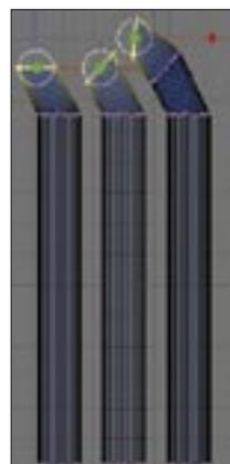
**Figure 4: Extruding means copying, moving, and rotating cross-sections. Blender uses the cross-sections to calculate the shape of the 3D object.**
