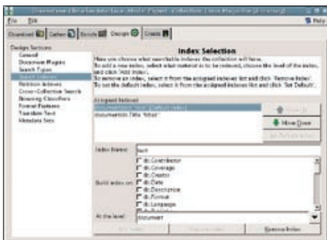
Figure 4: Define index settings in the Search Index section of the Design panel.
