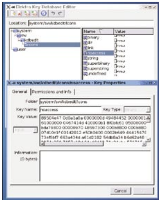
Figure 2: Elektra is designed to standardize Linux system configuration. The central XML file can be edited using a text editor, the KDB command line tool, or the KDBEdit front-end.
