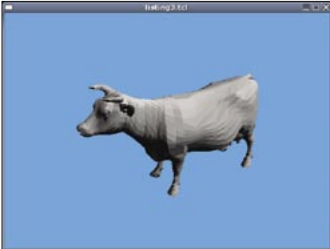
Figure 4: Instead of using a script to create every single element in a 3D model, OpenGL programs can load and display prebuilt 3D models.
