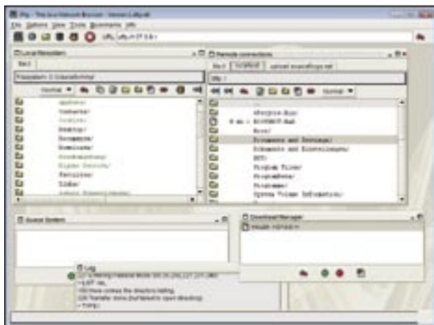
**Figure 1:** The Java-based JFtp client program gives Vista the ability to access NFS servers, along with SMB, FTP, or SFTP services.
